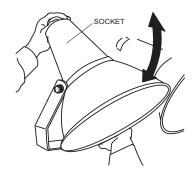
Figure 17. Adjusting Angle of Light
